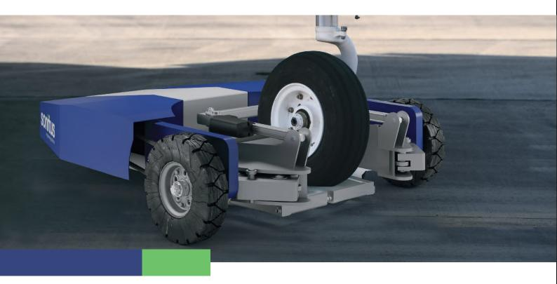
HATS provides high maneuverability to air vehicles within the tight spaces of the flight deck, ship's hangar, and a ground apron.
